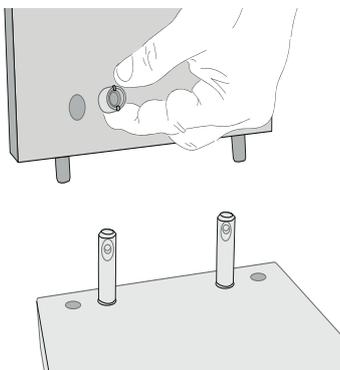
**1.** Screw the bolts into the side rails and insert the connector housing into head and foot sections. Align bolts and housing correctly!
