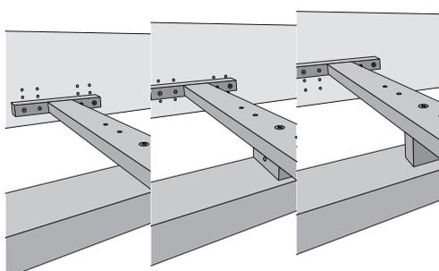
without spacer block: insertion depth 14,5 cm
