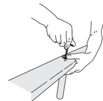
**6.** Choose the correct center feet and connect it to the center rail with the countersunk screw (M8x50). Mind the right length.
