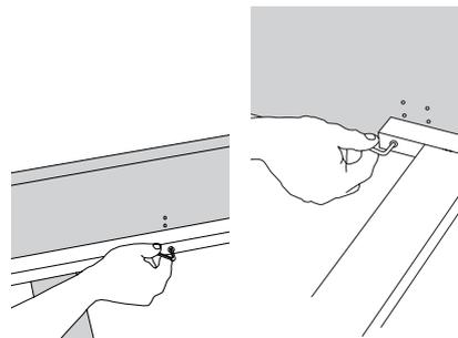
**5.** Fix the side supports using confirmat screws. For mattresses 140 cm or wider, fasten the center rail.
