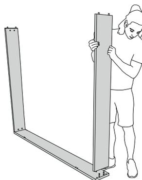
**2.** Attach the head and foot sections and fix them with grub screws.
