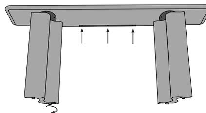
4. Move the console onto the mounting angle and fix it from below using Spax screws. If necessary, adjust the height-adjustable feet.
